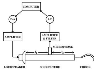
Figure 1. Schematic diagram of pulse reflectometer.
