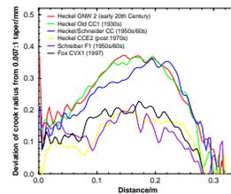
Figure 3. Six bassoon crook profiles plotted in terms of the deviation in radius from 0.007:1 taper.
